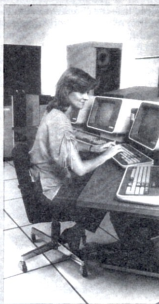
An IMI previewing system at Digital Productions calls up raster displays of simulated scenes on CRT monitors used for motion testing.
